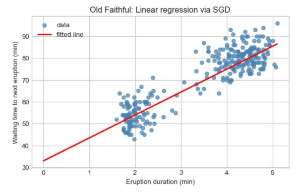
In the plot above, the line x=0 is included to facilitate the visualization of the intercept, which is given by  $\theta_0=32.910$ .
